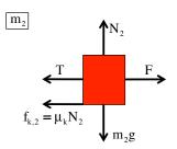
Notice I've used the same variable ("T") on each f.b.d. Why? Because the forces are action/reaction pairs and, as a consequence, have the same magnitude. ALWAYS DO THIS with action/reaction pairs!
